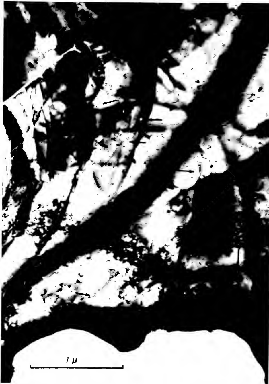
Figure 25.--Polyhedral voids in pulse quenched platinum foil after partial melting in the electron microscope. The average void size is approximately 300 \text{ \AA} .
